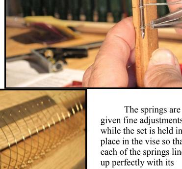
The springs are given fine adjustments while the set is held in place in the vise so that each of the springs lines up perfectly with its neighboring springs. Adjustments from sideto-side, and up and down are required to even out the line.
