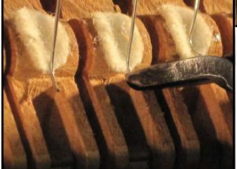
When the new set of hammer springs are reinstalled into the action of the piano, final adjustments are often necessary. Here, springs which are just a bit too long are clipped to the correct length, after which a new curved end is formed.
