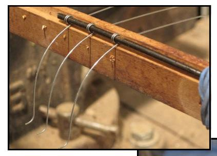
The tail of each new spring is then inserted though the original hole in the rail. (The short sliding wire helps keep the coils of the springs in line while the process is being completed.)
